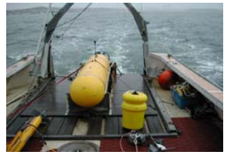
EdgeTech 2200-M Modular Sonar System installed on an AUV
